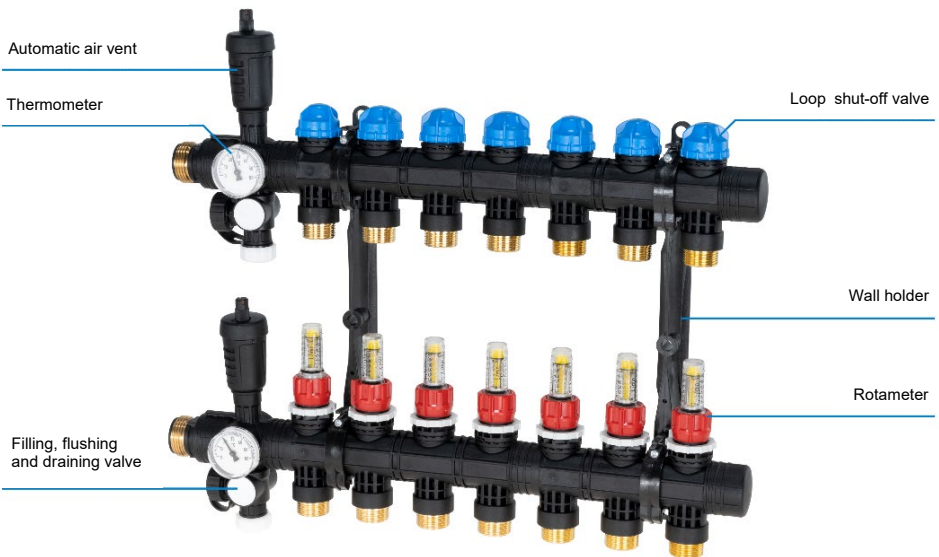
Figure 2: Construction of the ProCalida EF1 manifold
