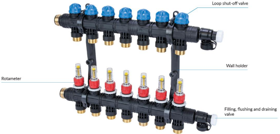
Figure 1: Construction of the ProCalida EF1 K manifold
