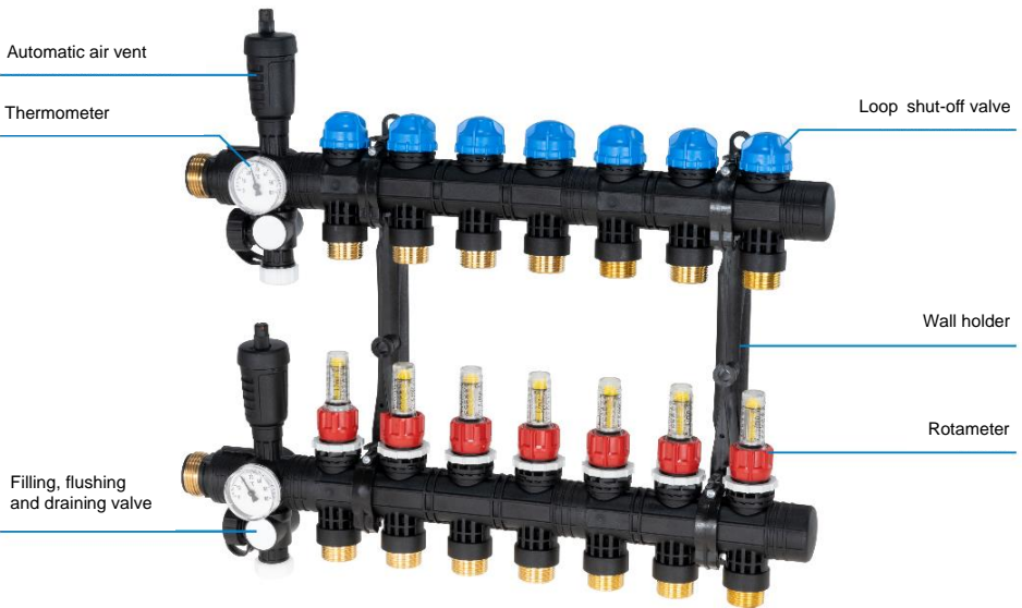
Figure 2: Construction of the ProCalida EF1 manifold
